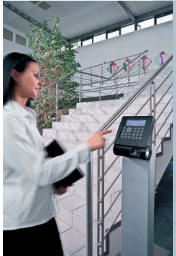
The IT8001 terminal is available for all standard identification media, such as proximity badges or key fobs, in all current reading technologies and also with optical fingerprint sensor.
